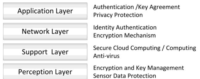
Figure 3. Four-Layer IoT architecture
