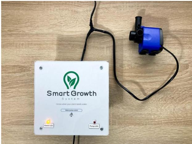
Figure 7. The watering pump component of the system
