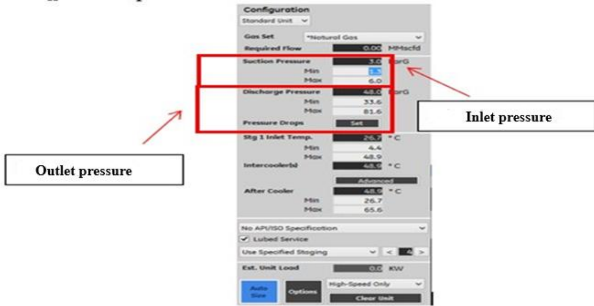
Figure 6: Input of Inlet and Outlet Gas Parameters
