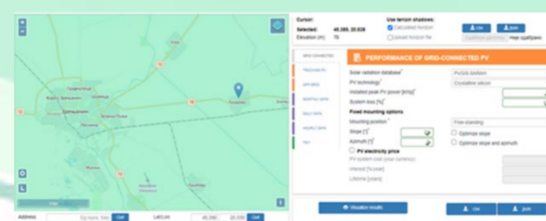
Setting of the location and angle of the receiver - 24^\circ in PV GIS
