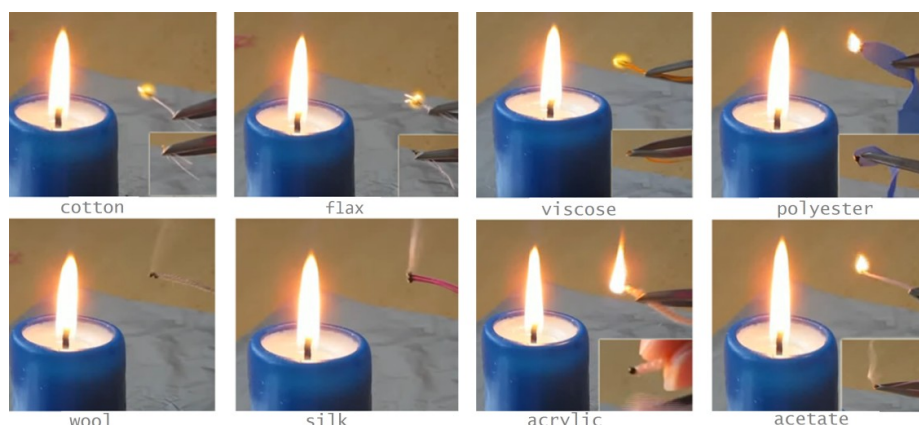
Figure 15: Burning Test for Textile Fiber Identification
