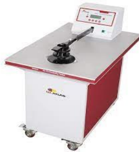
Figure 4: SDL ATLAS MO21A air permeability tester
