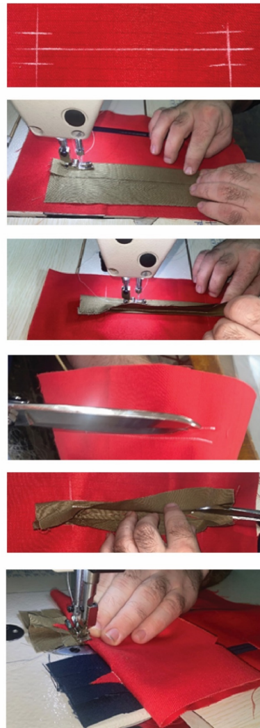
Figure 3. Method II of making a double welt pocket through phases
